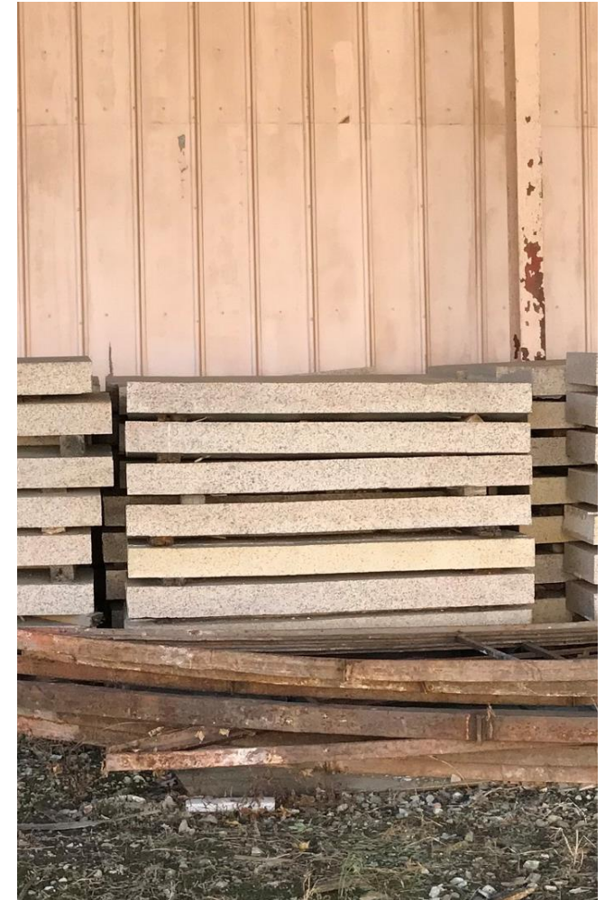
Salvaged 1974 Stair Treads
