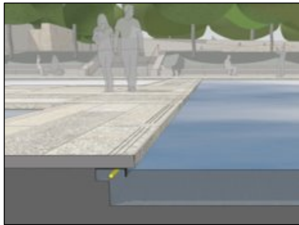
Proposed reflecting pool section with concealed safety and egress lighting. Black granite proposed for the 1974 pool and new reflecting pool.
