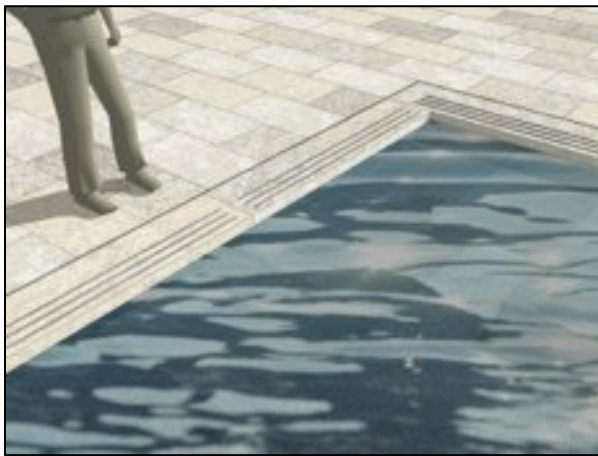
Proposed reflecting pool edge condition with Integral visual and tactile warning units.
